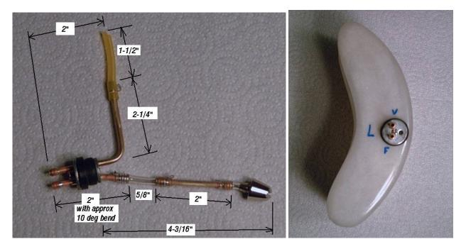
The main fuel tank has a capacity of approximately 60oz and is long and narrow so the internal plumbing arrangement is more typical. A length of brass tubing in the clunk line (similar to the 2" length of tubing used in the saddle tanks) will help prevent the clunk from falling to forward in the tank and will also limit the amount that the clunk line grows in length.
