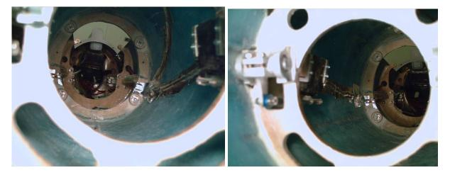
The aileron and flap servo wires are routed from the cutout in the wing root forward over the cutout for the gear strut. This area can become easily congested as several pneumatic lines route through this area. Ensure that the air lines and servo wires are routed such that they are not chaffed by the main wheels when the landing gear is retracted.
