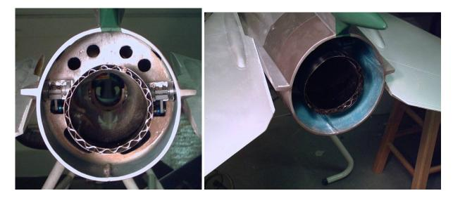
Apply several couple of coats of BVM Heat Shield to the aft area of the bypass. The upper portion of the bypass, if used, may be trimmed to suit the particular turbine installed and retained with Velcro straps.
