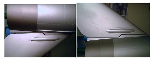
Portions of the root chord may be sanded down or build up using spot putty, as required, to adjust the H-stab root contour such that it matches the fuselage. This will allow the stabs to be installed with only a 1/32" gap between the stab and the fuselage which will enhance the look of your model. Use touchup paint to blend any spot putty visible. See "After" photos below.
