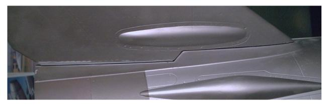
Cut away the vertical face of the notch at the fuselage root as shown below to allow the H-stab to rotate. This area is covered by the stab so it's not visible when the stabs are at neutral.
