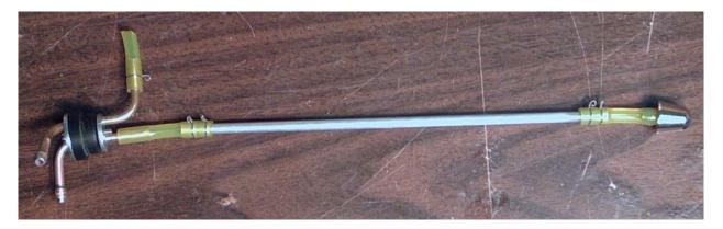
The forward face of the main tank, when installed in the model is quite close to the rear face of the cockpit. As such, a 90 degree bend in the fuel and vent lines prevents any interference between the lines and the cockpit.
